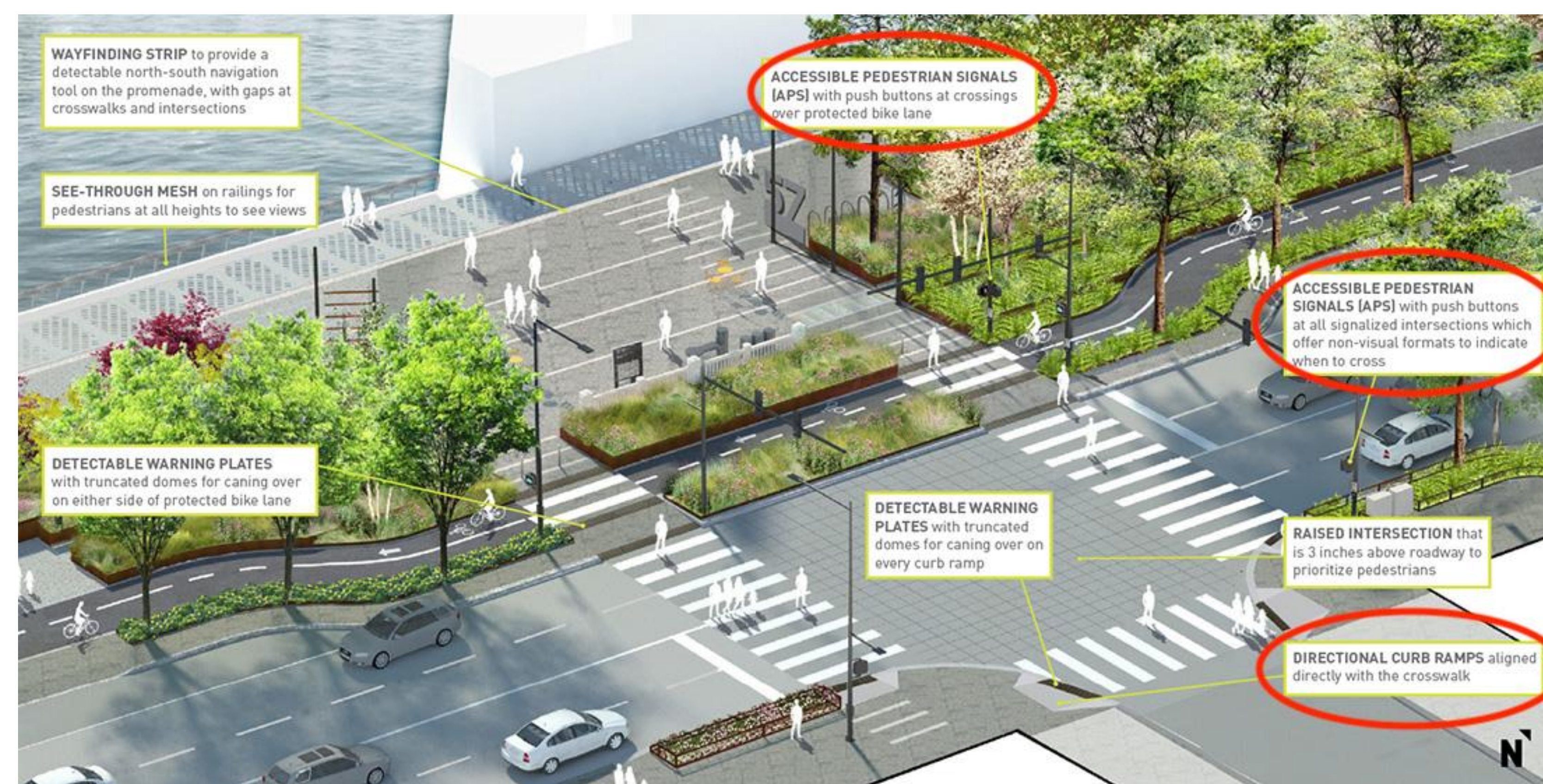
Figure 1: Rendering of a Seattle intersection with boxes pointing out various accessible figures. Red circles were added to denote the features discussed in our application: directional curb ramps and accessible pedestrian signals. 4
